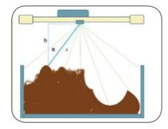
Each time the waste handling crane crosses predefined positions, either forwards or backwards, it carries out scanning and updates waste level of each position.
