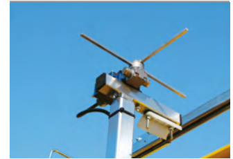
TROLLEY AND CRANE TRAVEL LIMIT SWITCHES
